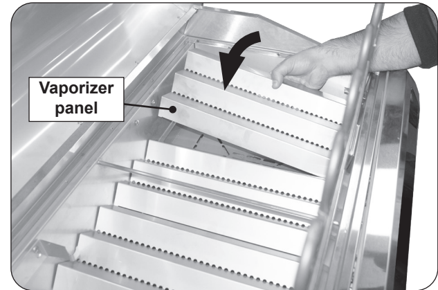
Fig. 34-2 Install vaporizer panels
