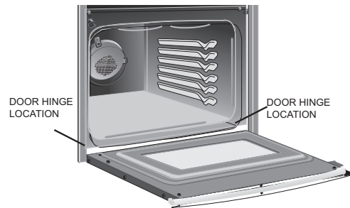
Figure 10: Door hinge location
