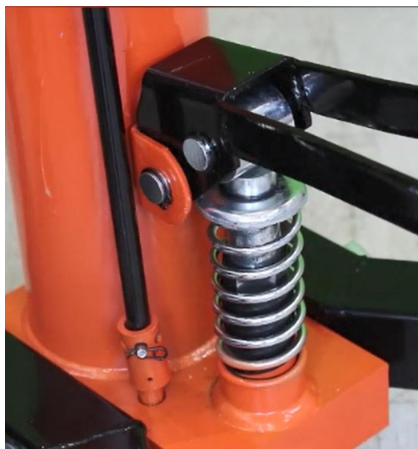
Step 5: Install handle ring screws.
