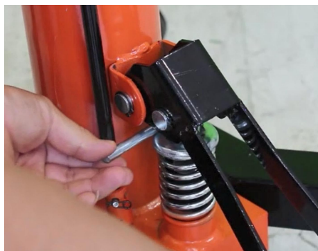
Step 4: Trap the handle over the cylinder.
