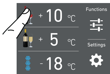
4) Home screen (*). - cantina compartment +8°C. - wine cellar compartment +5°C. - TriMode compartment -18°C.
