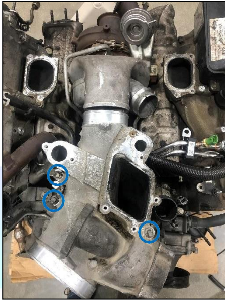
Figure 4: Lower Intake Bolts
