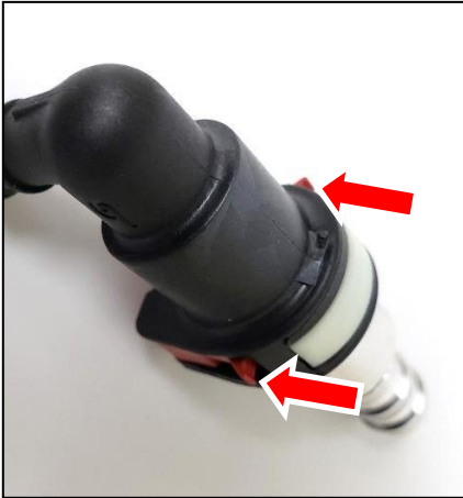
Figure 3: RED Lock + Push-Button QC – 2-step process
