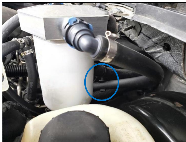
Figure 5: Zip tie clip placement
