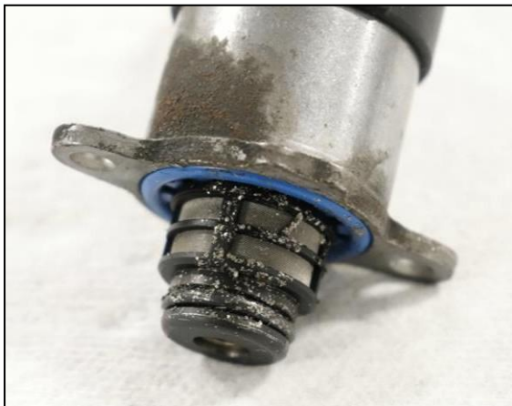
Figure 6: Failing CP4 FCA without Bypass Kit installed
