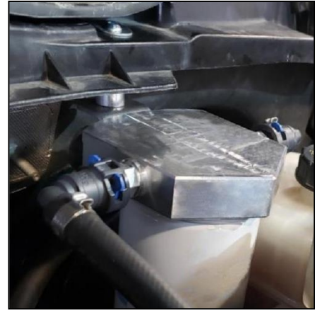
Figure 12: Filter Head Installed – 2017+
