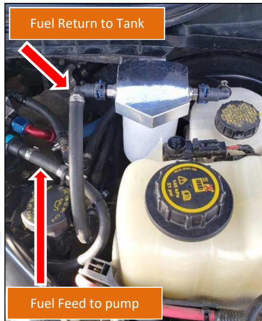
Figure 7: Left Side hose installation (2017+)
