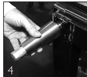
4 Thread leg into cabinet bottom frame rail.
