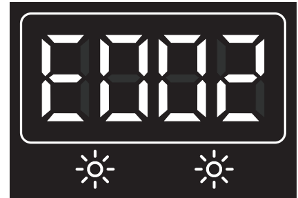
Figure 50 - Cascade System Error Code Example (Child Unit)
