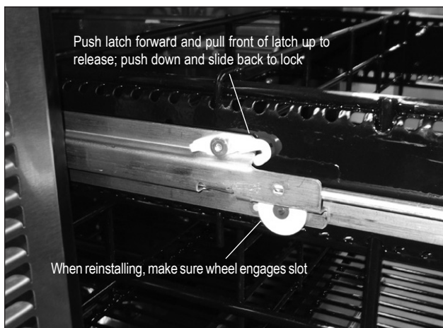
Figure 16: Removing/Installing Drawer
