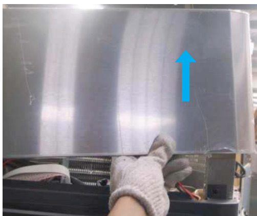
B. Lift top grille (T) as illustrated below.
