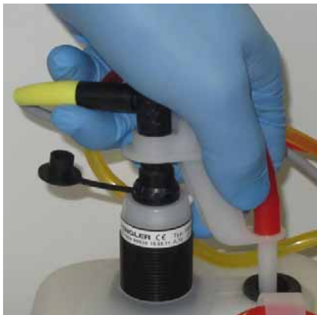
Figure 5–33: When pushing the tubing into the membrane, the connector is also plugged into the sensor
