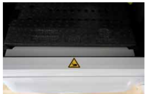
Figure 1–22: “Danger of crushing hands” right label
