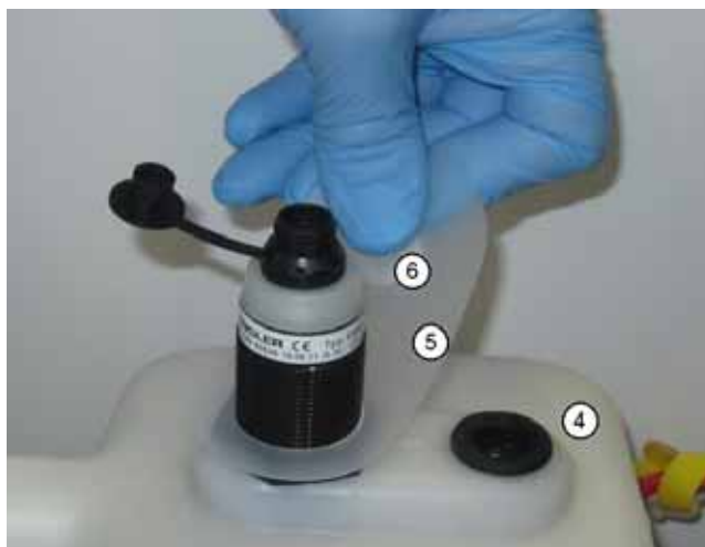
Figure 5–36: Rotation of the rubber strip and opening of the membrane
