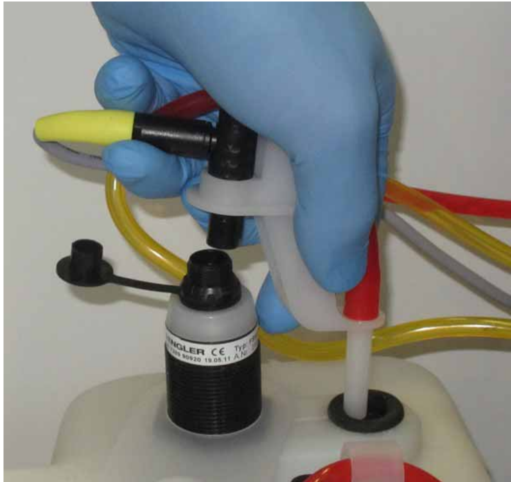
Figure 5–32: When unplugging the connector, the tubing is also pulled out of the membrane
