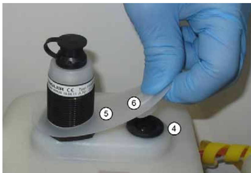
Figure 5–35: Rotation of the rubber strip and closure of the membrane with the cap
