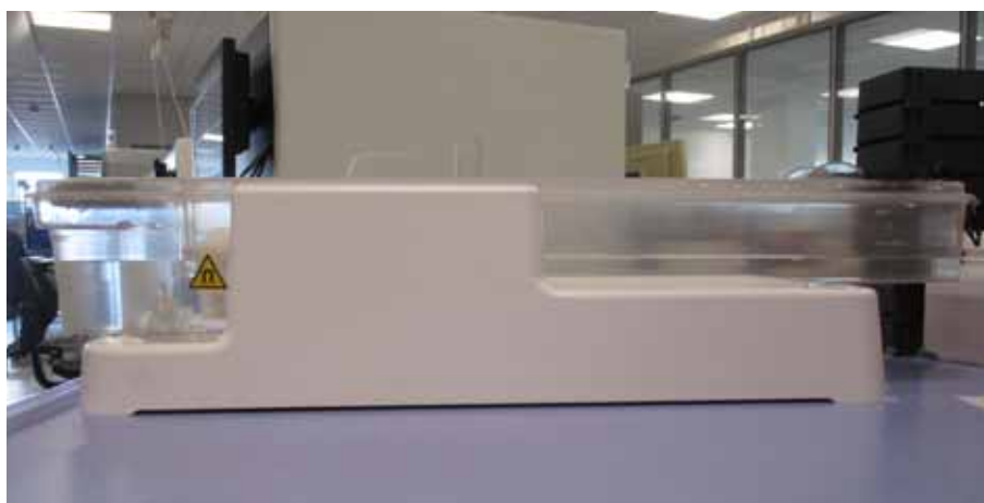
Figure 5-28: Preparation of Wash buffer - correct placement of the Wash Buffer tank
