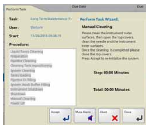
Figure 7–3: Long Term Maintenance - Manual Cleaning pop-up
