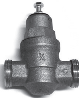
Figure 35: A Pressure Reducing Valve is required if your home's water pressure is above 80 psi.
