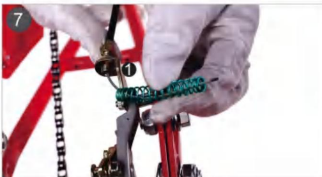
7. Put on the brake spring.
