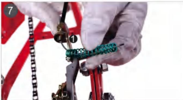
7. Put on the brake spring.
