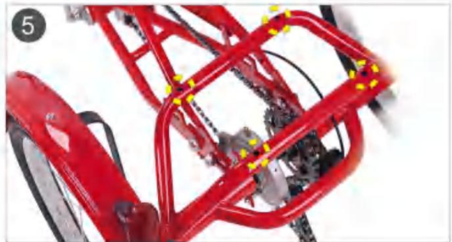
5. Four holes for fixing basket.
