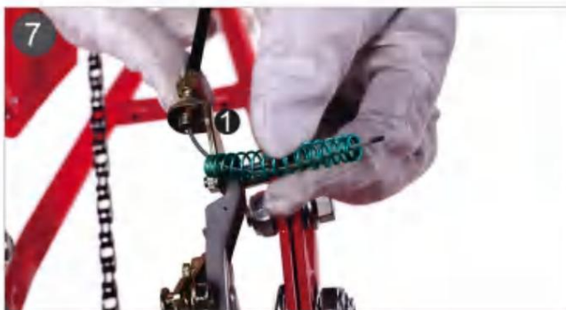
7. Put on the brake spring.
