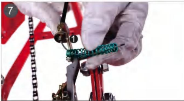
7. Put on the brake spring.
