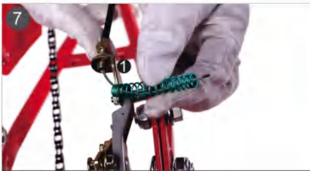
7. Put on the brake spring.
