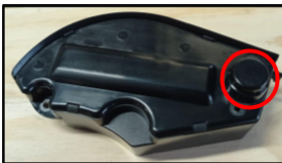
IoT box protecting cap circled in red
