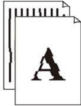
Lines Are Misaligned/Distorted
