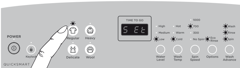
QuickSmart™ washer Customising a wash cycle, eg 'Regular' cycle
