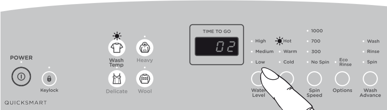
QuickSmart™ washer Adjusting the temperature setting, eg increasing the 'Hot' wash temperature by 2°C
