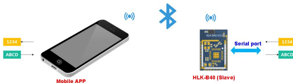
Figure 4 One-to-one Bluetooth connection transmission function schematic
