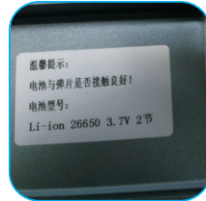
There is a tips of battery usage inside the battery compartment cover.
