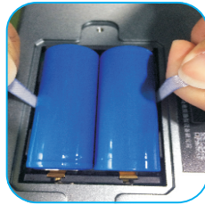
Take out the battery with both your hands Pull up the lifting rope pull up the lifting rope.
