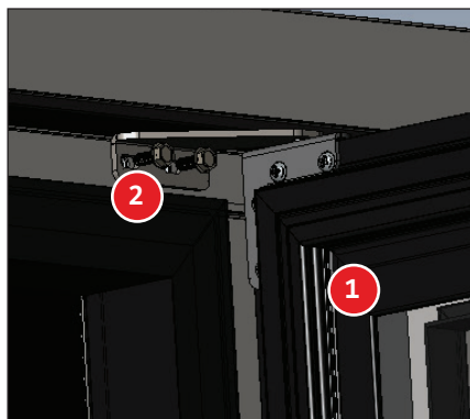
Fig. 10. Install the top hinge and the door.
