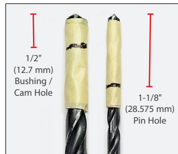
Fig. 8. Mark the hole depths on the drill bits.
