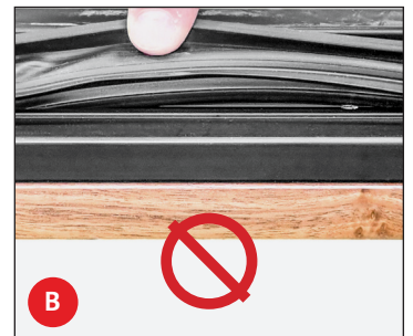
Fig. 12. Pull the side of the gasket to check its installation. A: CORRECT; gasket channel is NOT visible. B: INCORRECT; gasket channel is visible.
