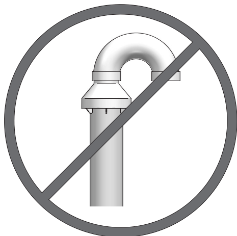
Figure 5-5 Do Not Install U-Bend to Rain Cap
