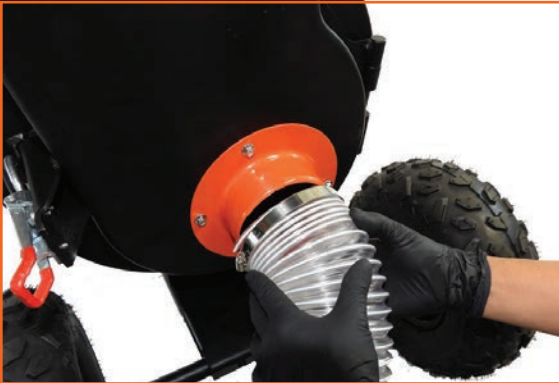
Install hose and hose clamp.
