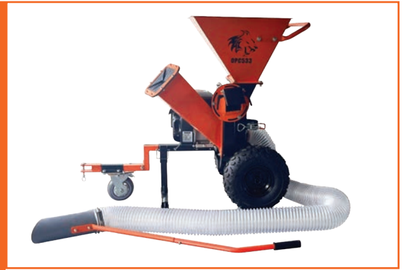
Run on high RPM with slide door closed to operate the vacuum.
