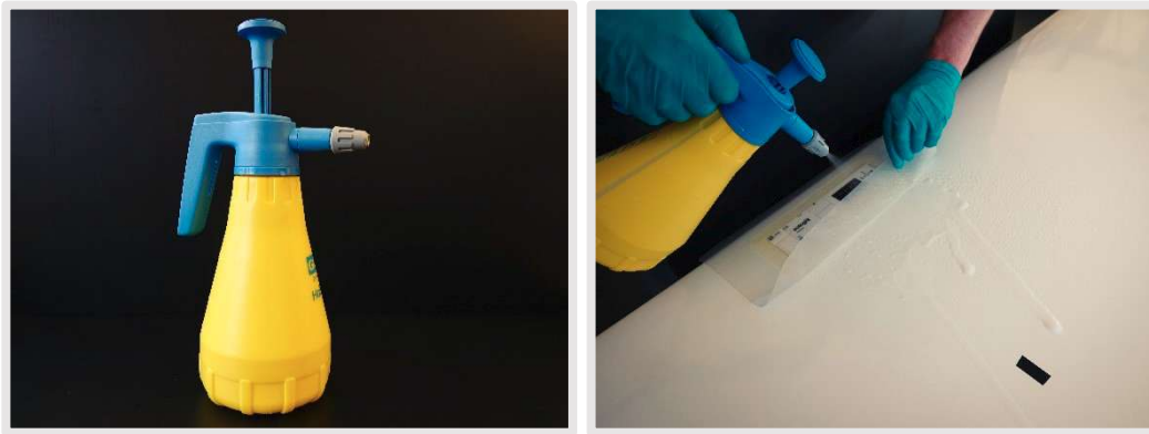
Figure 37 Apply assembly spray
