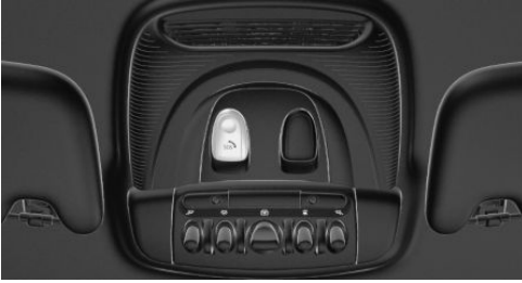
SOS button in the roofliner
