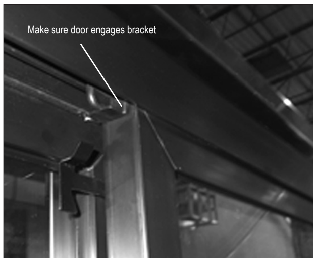
Figure 14: Removing/Installing Sliding Door
