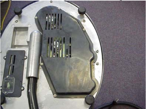
Figure 10. Cover over blender drive system.
