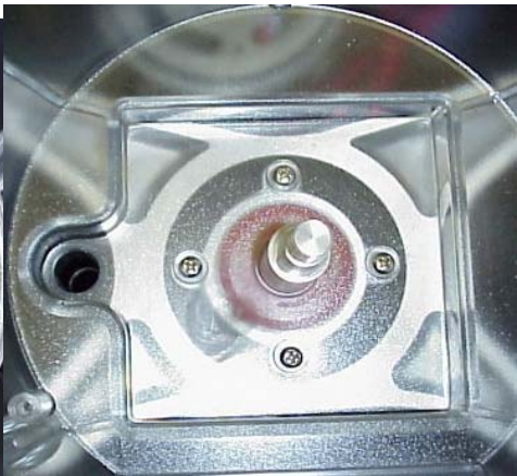
Figure 4. Clean Drain Pool
