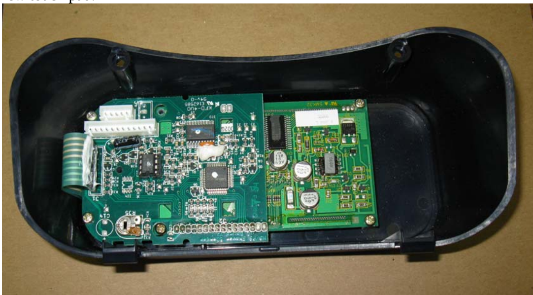
Fig. 21. Rear of Control Panel removed from unit.
