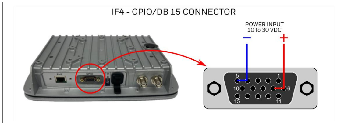
Fig. 6 – Powering IF4 with external DC power supply.
