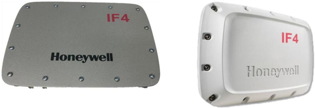
Fig 1- IF4 a) Without integrated antenna. b) With integrated antenna.
