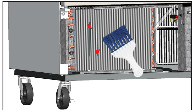
Fig. 4. Never brush across the coil fins.
