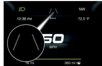
Lane Markings Not Detected
