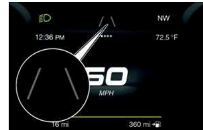
Lane Markings Not Detected
