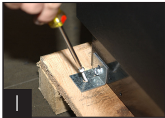
1 Removing bracket from skid.
