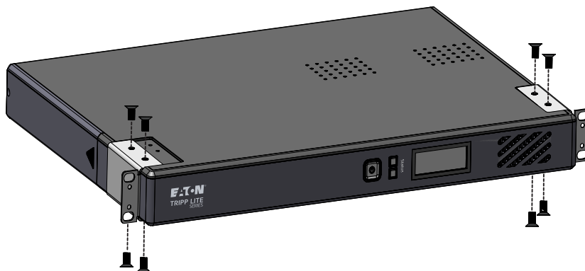
Figure 7. Four Post Rack Installation
