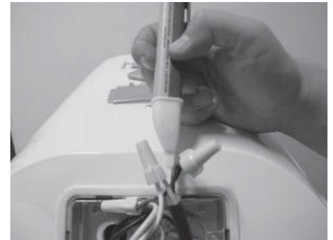
Figure 28 - Non-Contact Circuit Tester
