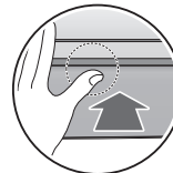
<Lock the bottom hook>
