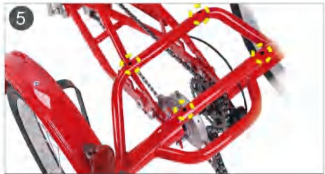
5. Four holes for fixing basket.
