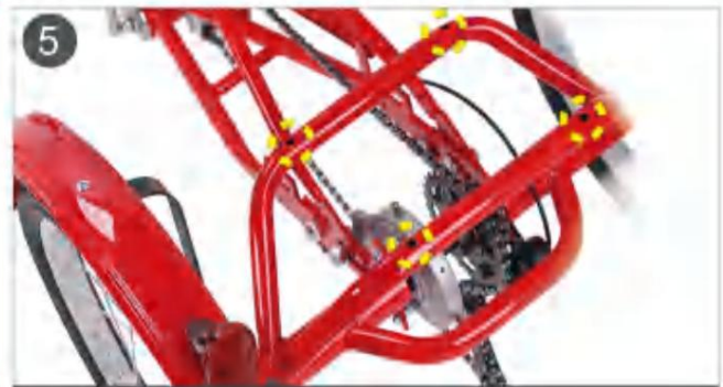
5. Four holes for fixing basket.
