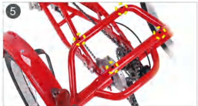
5. Four holes for fixing basket.
