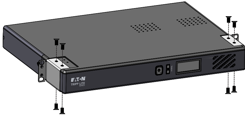
Figure 8. Two Post Rack Installation
