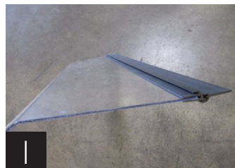
Air deflector and hinge assembly
