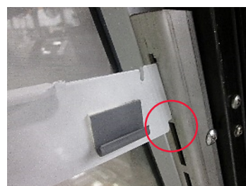
Top notch installed (gap)
