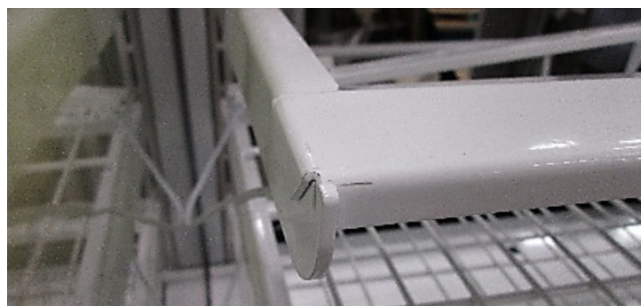
Light assembly installed on shelf support
