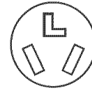
3-wire receptacle (10-30R)
