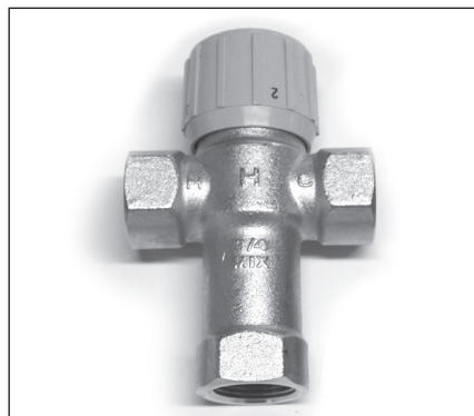
Figure 24 - Adjust Thermostat Mixing Valves at each point-of-use to 120°F/49°C or lower.
