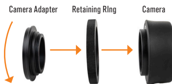
Fig. 7: The camera adapter goes through the retaining ring and threads into the bottom of the camera.
