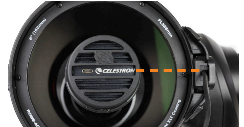
Fig. 9: We recommend orienting the camera as shown, with the sensor parallel to the Celestron logo on the front of the camera. This positions the sensor perpendicular to Origin's altitude axis.
