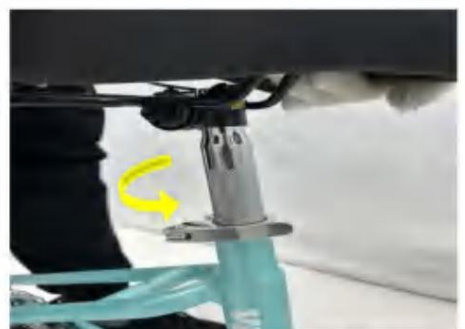
Adjust the height and Angle of the saddle and tighten the saddle clamp
