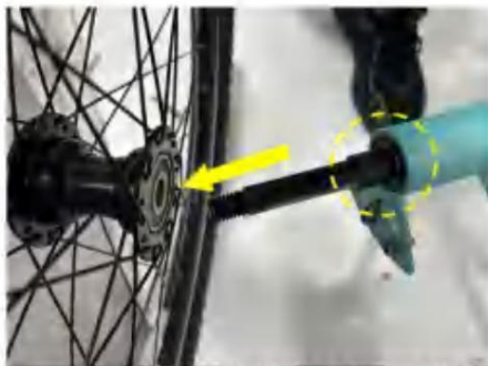
Insert the rear tripod shaft to the left/right Side Wheel (note the sleeve of the yellow circle)
