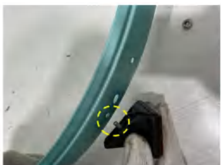
Insert the rear reflector screw into the hole as shown
