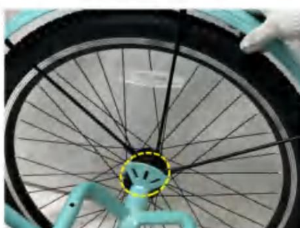
Note that rear fender support rod holes correspond to frame holes
