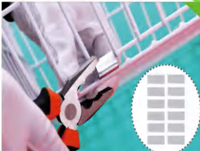
Secure with metal sheets
