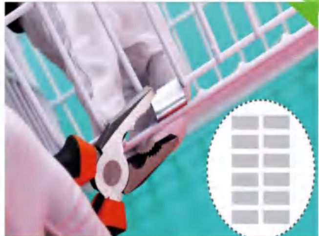
Secure with metal sheets
