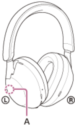
A: Location of the built-in antenna
