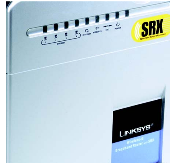
Figure 3-3: The Router's LEDs
