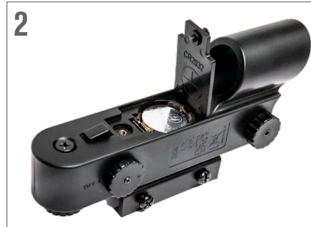
2. If you are replacing the battery, install the new one with the (+) terminal facing outward.
