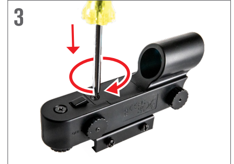
3. Place the cover back onto the finderscope and retighten the screw with the Phillips-head screwdriver.
