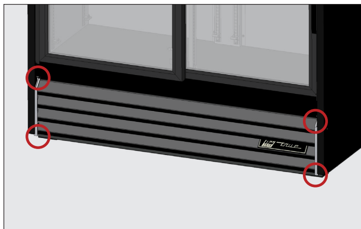
Fig. 2. Slide door louver grill screw location.
