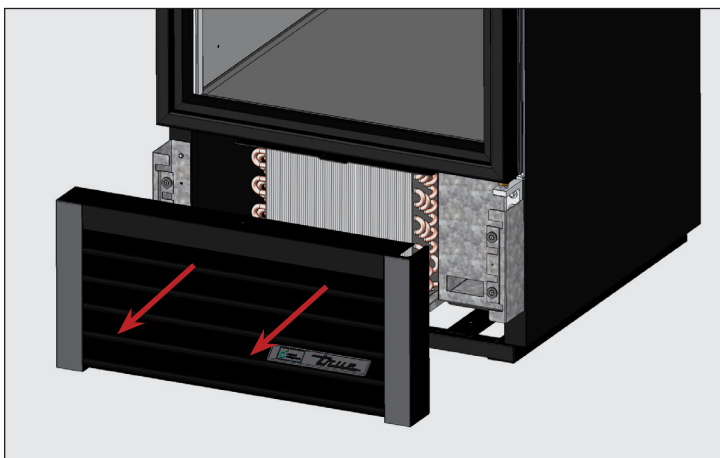
Fig. 3. Carefully remove the grill.
