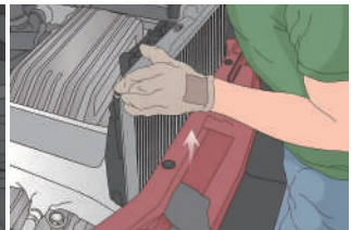
Lift out the radiator
