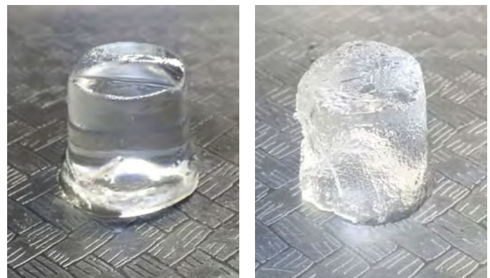
FIG. 2. Ice deteriorates and roughens as it ages.
