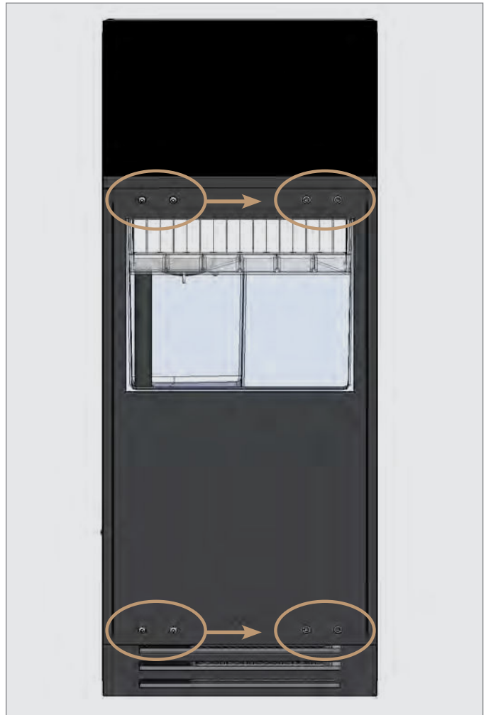
FIG. 8. Move the remaining door hardware to the opposite side.
