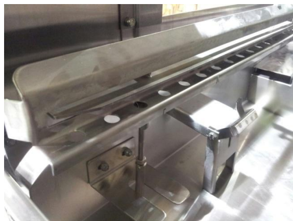
Wash tank sequence bar, pendulum with magnet
