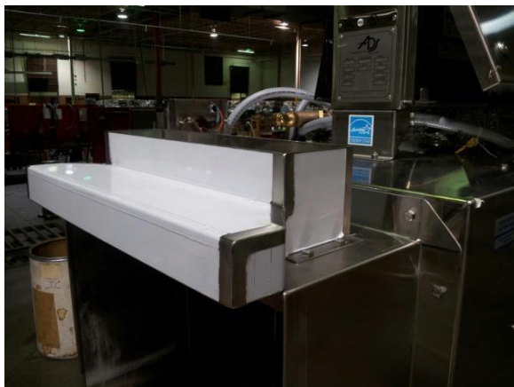
Vent attachments to end shield, 4" x 16" opening
