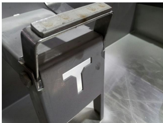
Showing wash arm T index for lower arm
