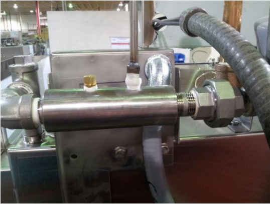
Mixing chamber with two 1/8" pipe threaded ports Hi-temp mixing chamber is SS, Chemical is a polymer
