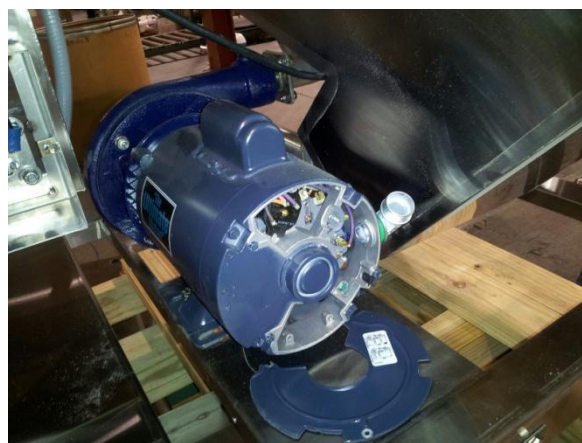
66 power scrapper motor, 1.5 HP, 208v, single-phase
