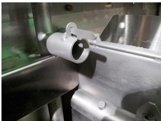
Showing pumped rinse manifold locking tab
