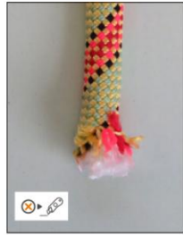
• Damaged rope end
