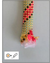
• Damaged rope end
