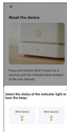
③ Press and hold the Reset button for 5 seconds until the Wi-Fi indicator blinks; then select the status of the indicator light
