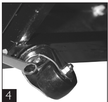
Tighten castor in position with castor wrench.
