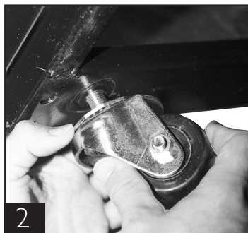
Thread castors into existing leg leveler holes.
