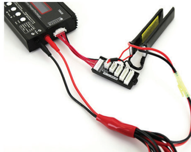
Balance charging / storage / discharge mode
